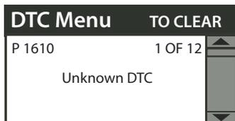
On this screen, scroll down to view all DTCs. Press "Y" to erase the DTCs, Press "N" to exit back into the main menu without erasing the codes.
