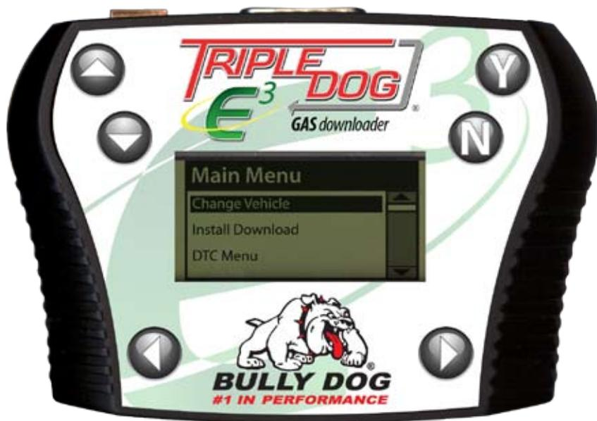
**CHANGE VEHICLE:** Select this option to navigate to the Vehicle Selection screen and choose a new vehicle type.
